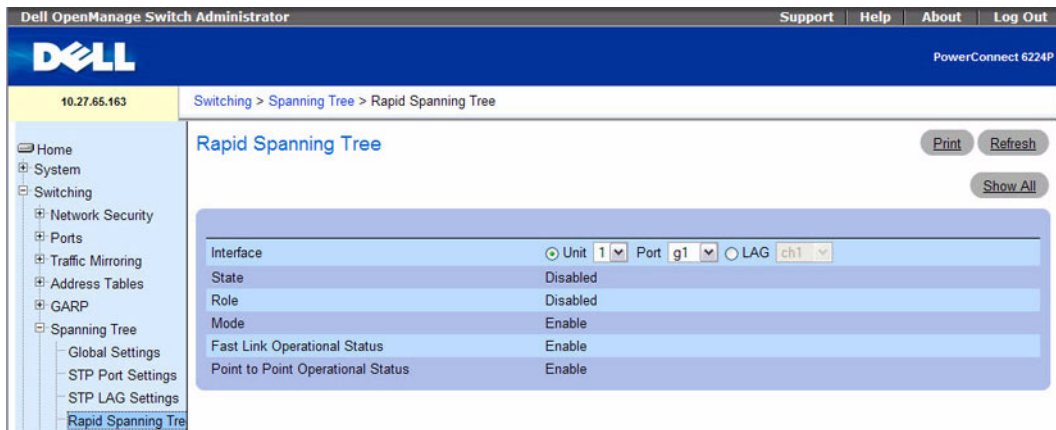
Figure 7-43. Rapid Spanning Tree
